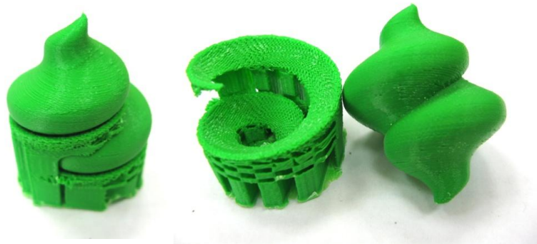
Example of a stable support during printing for the reachable set
