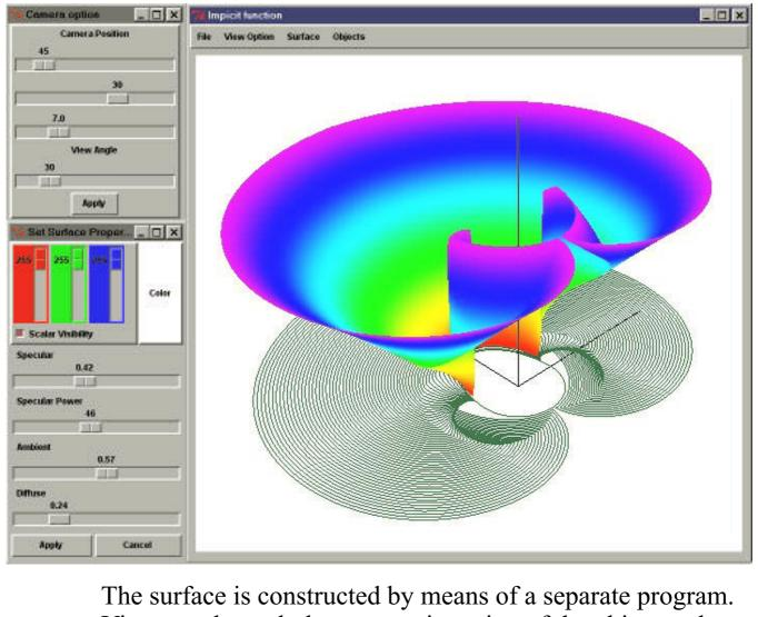
The surface is constructed by means of a separate program. Via control panel, the space orientation of the object and its coloring can be changed. Both the surface and its level lines are shown.
