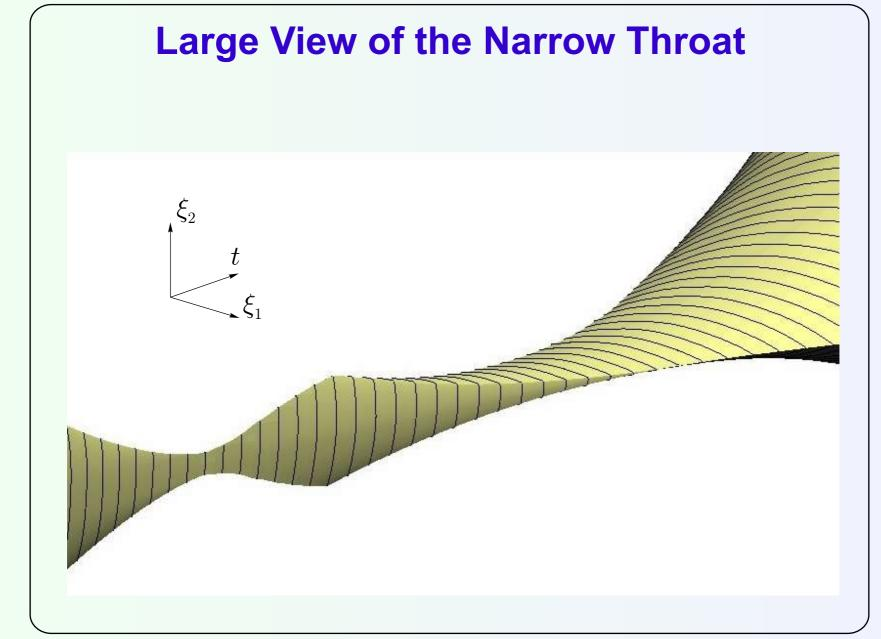
This is a large view of the throat. The time sections of the tube are convex, but their geometry is changing in time non-trivially. This is the result of numeric computations. It is very difficult to give analytical description of the value function in this region.
