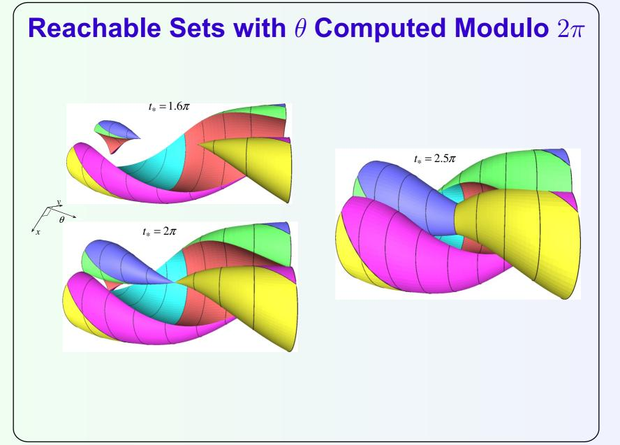
It is possible to pass to the sets, for which the angle  $\theta$  is calculated modulo  $2\pi$ . This slide shows such sets for three instants. When demonstrating such three-dimensional reachable sets to students, we emphasize that the Pontryagin maximum principle is only a necessary condition for the control leading a non-linear system to the boundary of the reachable set.
