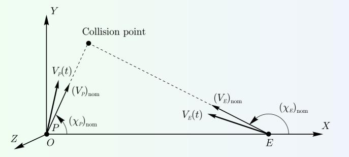
$$\begin{aligned} \ddot{x}_P &= a_P, & t \in [0, T], \quad x_P, x_E \in \mathbb{R}^2, \\ \dot{a}_P &= (u - a_P)/\tau_P, & u \in P, \quad v \in Q, \\ \ddot{x}_E &= v, & \varphi \left( x_P(T), x_E(T) \right) = \left| x_E(T) - x_P(T) \right|. \end{aligned}$$
