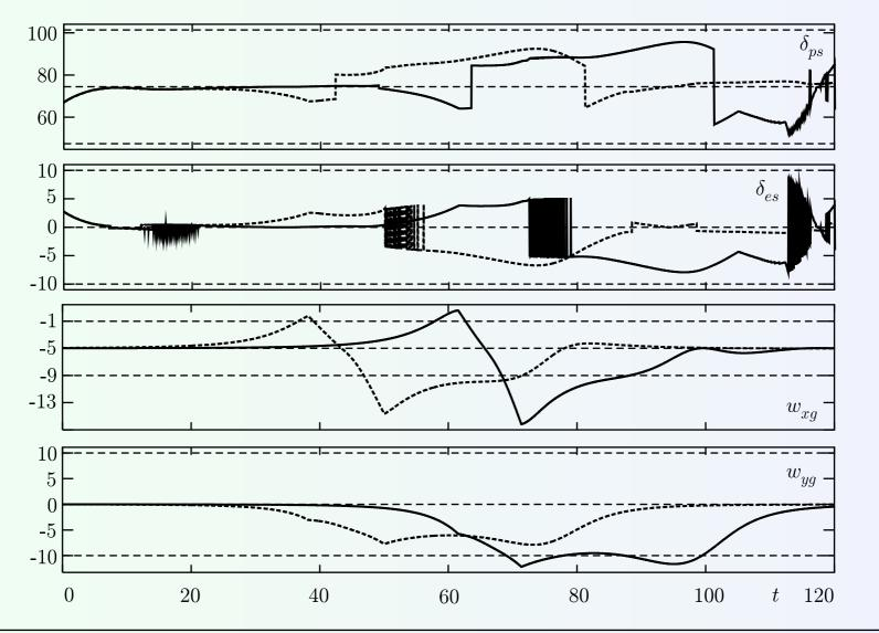
On this slide, we see the realizations of the thrust and elevator controls. These are command control signals. Below, the realizations of longitudinal and lateral wind disturbances are shown. They were created by means of a wind microburst model. We used two variants of the location of the microburst zone.
