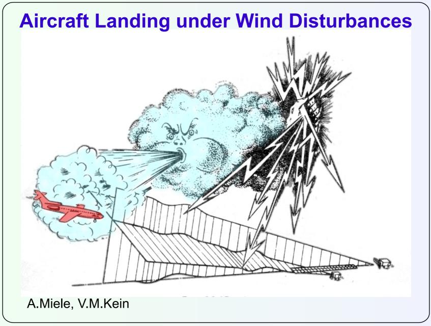
The problem of aircraft landing under wind disturbances is the natural example for mathematical control theory and differential games. But there are some difficulties for formalization of such a problem as a differential game. Namely, the aircraft has four main controls: thrust, elevator, rudder, and ailerons. Bounds for their ranges are known. Therefore, we can strictly describe the constraints for the useful control. In contrast, we do not know the real constraints for the wind disturbances.
