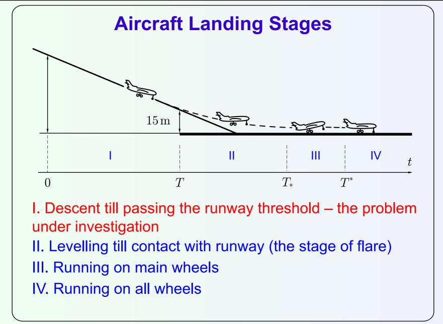
In our investigations, we consider the part of the landing process from the height about 400 meters till passing the runway threshold at the height about 15 meters, that is, the part when the nominal trajectory of the aircraft is a rectilinear glide path.
