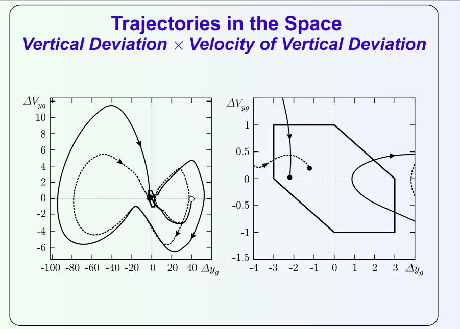
Here, the results of simulations of the non-linear system for two variants of the wind disturbances are given in the variables of the vertical channel. We see phase trajectories in the plane *vertical deviation from the nominal motion*, the velocity of the vertical deviation. At the right, we see a large view of the area near the terminal target set. The polygonal target set is the tolerance for the vertical channel.
