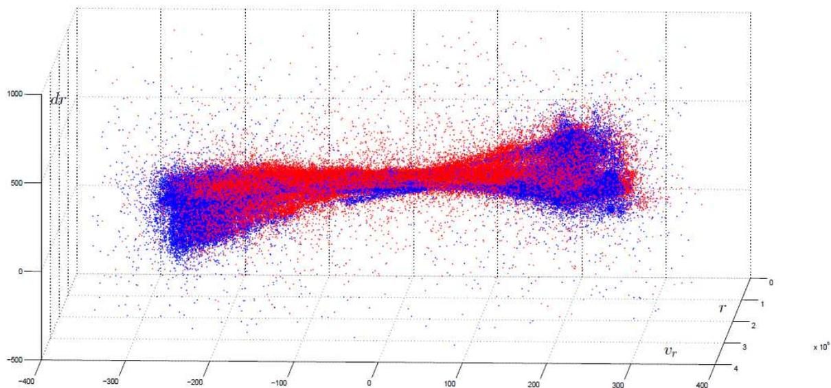
Figure 3. A three-dimensional graph of the dependency of  $dr$  on  $v_r$  and  $r$  for the radars at the site 1. The linear connection of the  $v_r$  level and divergence in  $dr$  is clearly visible. The values of  $dr$  and  $r$  are specified in m,  $v_r$  are specified in m/s
