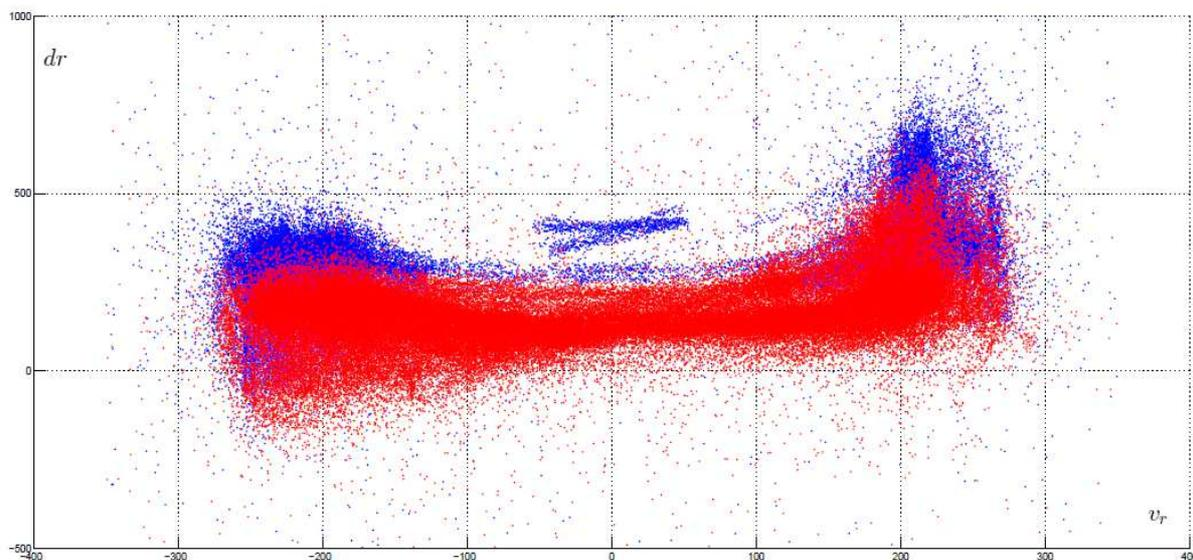
Figure 2. The graph of the dependency of  $dr$  on  $v_r$  for the radars at the site 1. The values of  $dr$  are specified in m,  $v_r$  are specified in m/s
