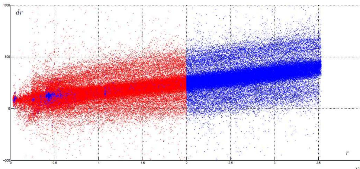
**Figure 1.** The dependency of  $dr$  on the range  $r$  for radars at the site 1 in Moscow ATC zone. The measurements of SSR are blue, the measurements of the combined radar are red. The values of  $dr$  and  $r$  are specified in m
