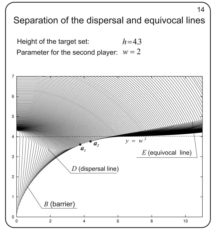
On this slide, a fragment of the collection of the level sets is shown for h = 4.3. One can see the curve composed of the corner points of the fronts is divided onto two parts. For *h* cosidered, the division point  $a_1$  and  $a_2$  are close to earch other.
