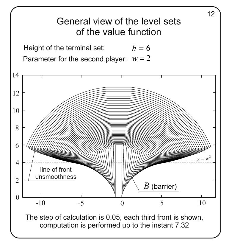
Here, level sets of the value function are presented for h = 6, w = 2. The curve consisting of the corner points of the fronts is clearly seen. This curve coincides with our singular line. The region that is filled out with the fronts coincides with the solvability region. The accumulation of the fronts near the horizontal line  $y = w^2$  means that the value function goes to infinity when approaching  $y = w^2$  from above.
