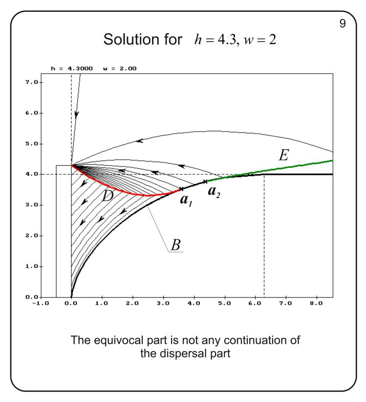
If *h* decreases further, the singular line breaks up: the dispersal arc approaches the barrier *B* tangentially at the point  $a_1$ , but the equivocal arc emanates tangentially from another point  $a_2$  lying on the barrier on the right from the point  $a_1$ . Basically, the singular line consists of three parts as before.
