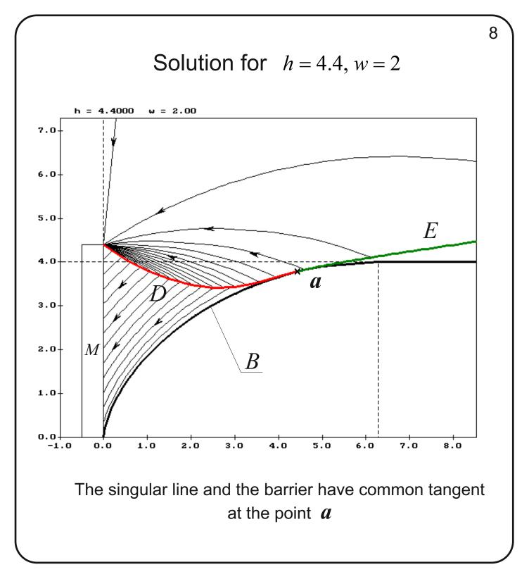
If h continues to decrease, the singular line approaches the barrier line near and near. The limiting case where the singular line touches the barrier is shown.
