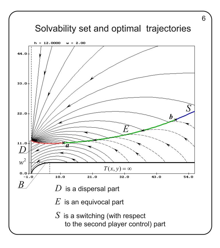
The singular dispersal line D was computed from the condition that the attainment instants along characteristics of the first and second families are equal. Parts of characteristics computed backwards are removed beyond intersection points with D. Each point of D is a source for two optimal trajectories. The construction of the dispersal line is stopped if it becomes tangent to one of the trajectories of the first family. A point corresponding to this situation is denoted by a on the slide.
