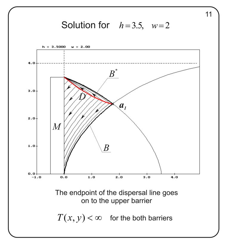
If h decreases, the solution structure remains the same: two barriers define the solvability region. The endpoint of the dispersal arc goes on from the lower barrier to the upper barrier. The value function is finite on both barriers.
