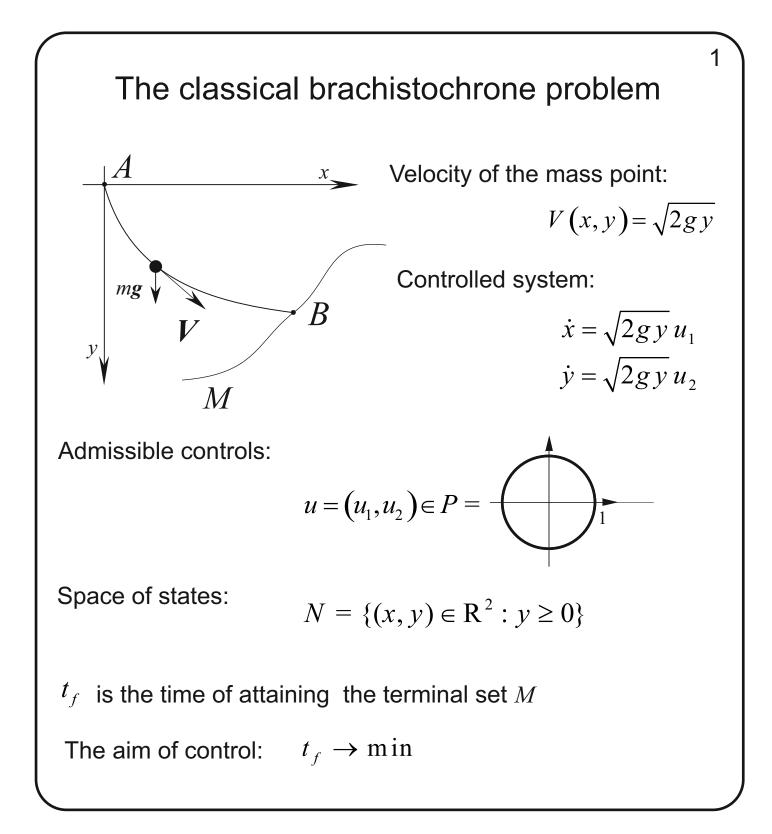
Let *A* and *B* be arbitrary points in the vertical plane. One looks for a curve connecting *A* and *B* such that a massive point being started from *A* with zero initial velocity attains *B* along this curve for the minimal time. In the general case, the terminal point *B* is replaced by a given terminal curve *M*. For any trajectory, the velocity of the mass point at (x, y) is  $(2gy)^{1/2}$ , where *g* is the gravitation constant.
