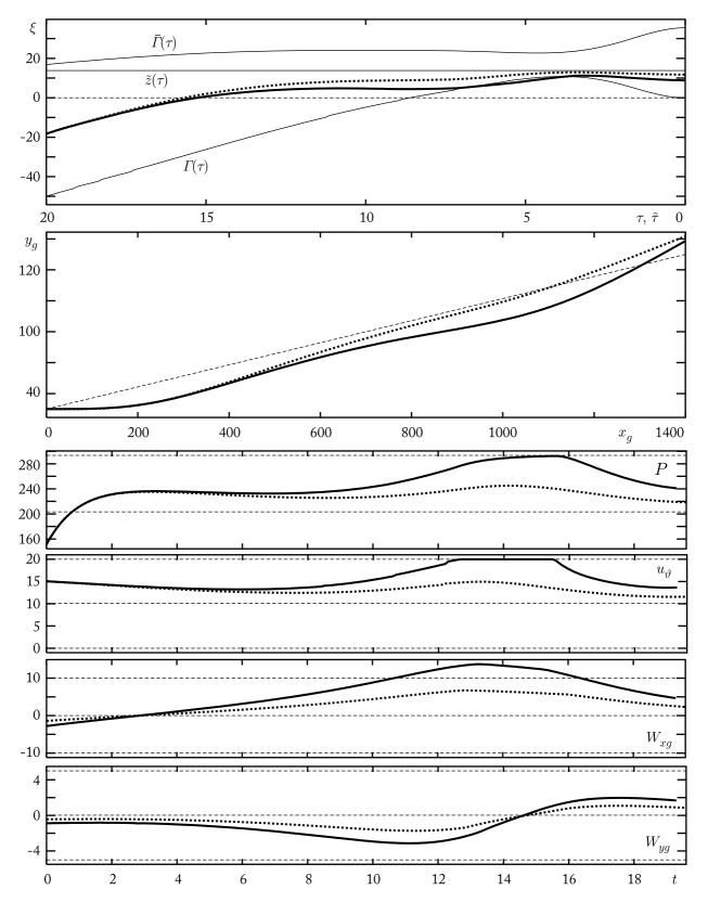
Fig. 5. Simulation results; the plane of auxiliary game (4) in the upper fragment; below that fragment, the graph of the altitude; the graphs of the thrust force P (×1000 N); the prescribed pitch angle  $u_{\vartheta}$  (grad); the longitudinal  $W_{xg}$  (m/sec) and vertical  $W_{yg}$  (m/sec) components of the wind velocity
