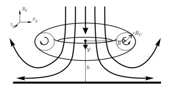
Fig. 4. Wind microburst model
