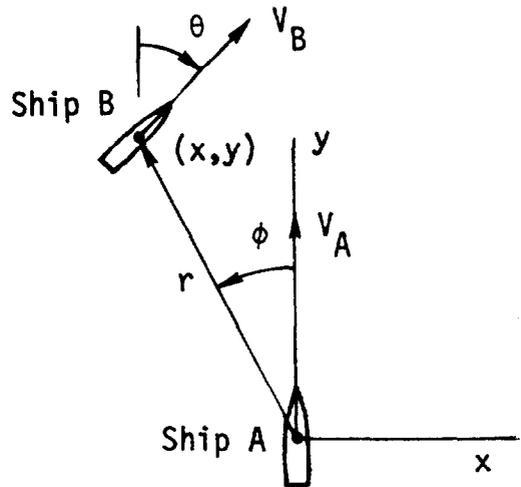
Fig. 2—Geometry of the Two-Ship Encounter.
