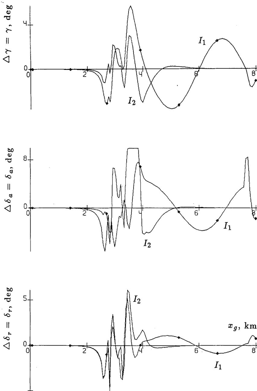
Fig. 7d. Deviation histories: bank angle  $\gamma$ , aileron deflection  $\delta_a$ , rudder deflection  $\delta_r$ ; Model M2, downburst center  $DY = 3000$  m,  $DZ = 200$  m.
