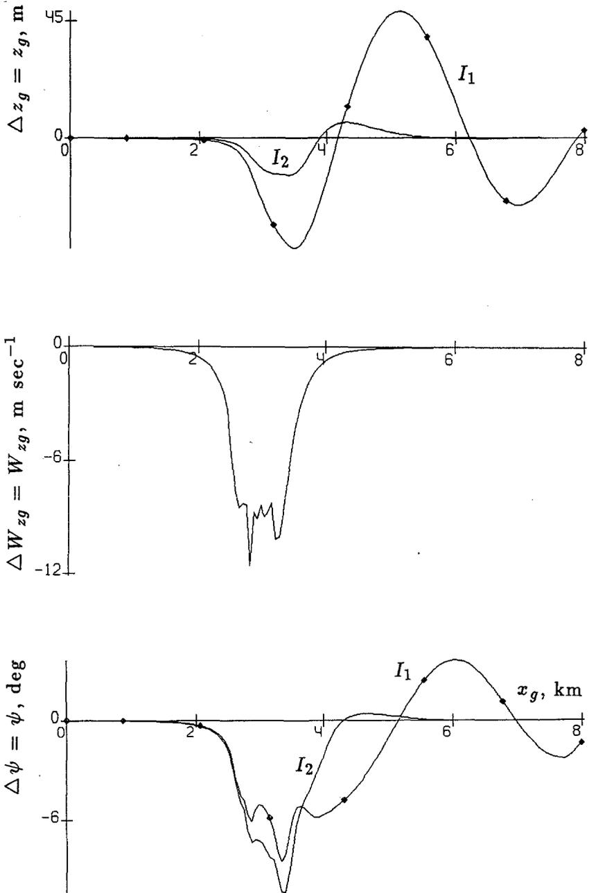
Fig. 7c. Deviation histories: lateral position  $z_g$ , wind velocity component  $W_{zg}$ , yaw angle  $\psi$ ; Model M2, downburst center  $DX = 3000 \text{ m}$ ,  $DZ = 200 \text{ m}$ .
