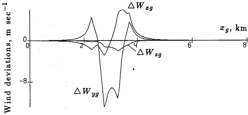
Fig. 4a. Landing simulation results for Model M1; downburst center  $DX = 3000$  m,  $DZ = 100$  m.
